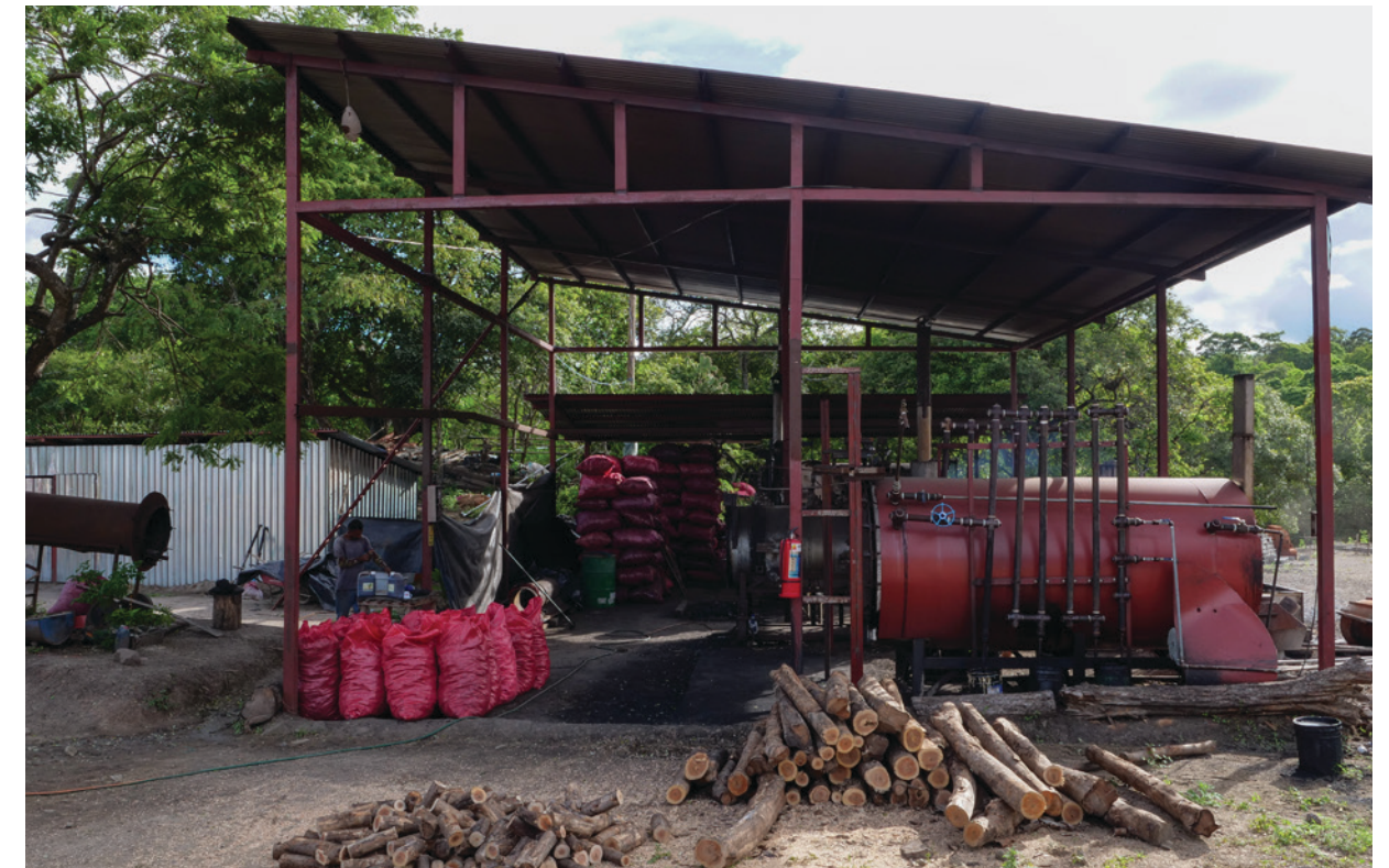
A biochar reactor at CommuniTree's production centre helps deliver long-term livelihood opportunities for farmers.
